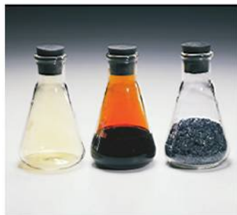
▲ FIGURE 9-13 Three halogen elements Chlorine is a yellow-green gas. Bromine is a dark red liquid. Iodine is a grayish black solid.
