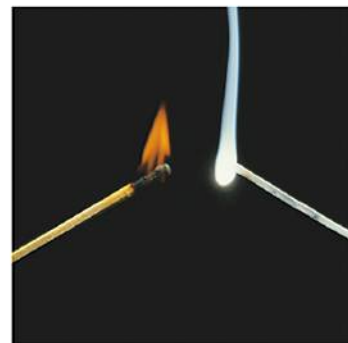
▲ FIGURE 2-1 Two combustion reactions The apparent product of the combustion of the match—the ash—weighs less than the match. The product of the combustion of the magnesium ribbon (the “smoke”) weighs more than the ribbon. Actually, in each case, the total mass remains unchanged. To understand this, you have to know that oxygen gas enters into both combustions and that water and carbon dioxide are also products of the combustion of the match.
